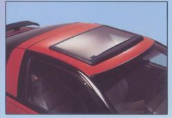
An aerodynamically designed wind deflector improves airflow and reduces wind noise.
