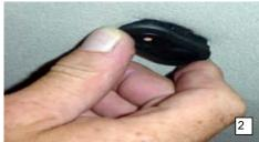
Disengage the switch from the headliner/trim ring.
