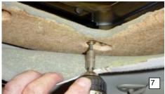
Remove enough screws so the bezel can be deflected downwards, to gain access to the motor assembly. (450 HS only)
