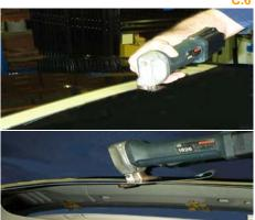
Using an air chisel, cut a starter hole approximately 3" in diameter in the center of roof opening.
