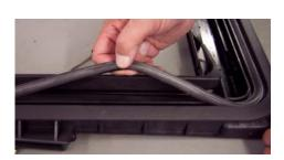
Insert the new seal, starting in the four corners. equally dividing the seal.
