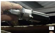
Remove the motor assembly.
