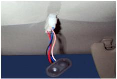
Install the headliner into the vehicle.
