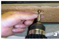
Remove the T-25 screws retaining the bezel to the mainframe. (450 HS only)
