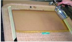
Pre spray glue to the leading edge for headliner retention.
