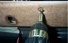
Install substrate to the mainframe using a T-20 torque bit driver.
