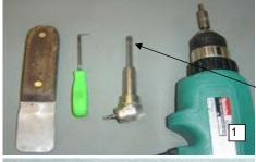
Tools required to remove the SCU & motor.
