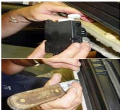
Unplug the motor connector from the SCU and replace the SCU.
