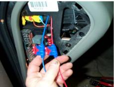
Route the harness wires down the A-post. Tape the wires into place.
