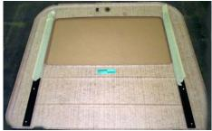
Tape the track guides with masking tape to avoid prolonged clean up.
