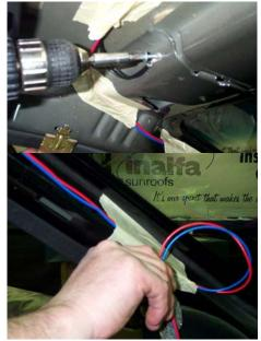
Connect the ground wire to the front header.
