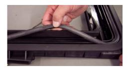
Remove the seal section from the mainframe.
