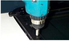
Remove 4 screws retaining the lower clamp frame to the mainframe. Remove 1 motor screw, the Motor remains in place.
