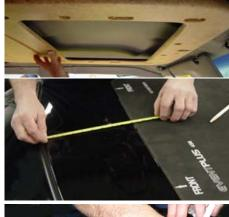
From outside the vehicle locate the up ding and measure 2 1/4" forward and mark. Align the front edge of the cutting template with the mark.
