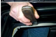
Tuck the material using a tucking tool.
