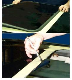
Pre-fit the Spoiler unit into the roof opening to insure that the opening is a minimum of 1/16" larger than the mainframe.
