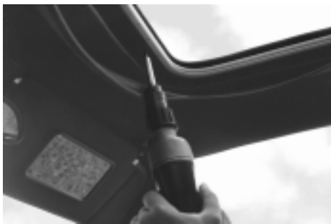
Step 11 - installation of trim ring
