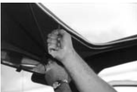
Step 9 - cutting headliner board
