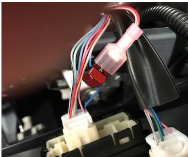
Picture 31B: Red-white wire connected to blue wire.
