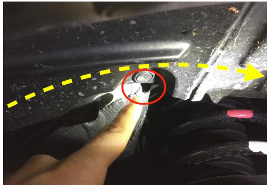
Picture 19: Yellow lines show the wire harness path.
