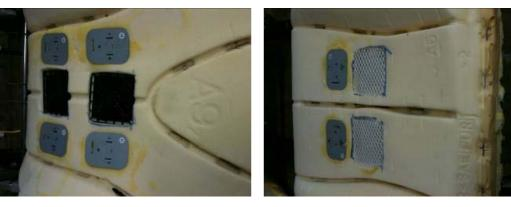
Make sure the cooling fan is located inside the cushion and cover it with one piece of perforated spacer. This is so that the customer will not feel the fan when sitting on top of the cushion.
