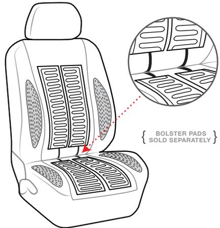
**NOTICE :** If you are installing bolster pads ONLY, the connections will remain same. Ignore the connection to regular heat pads and secure all loose wires and connectors. Do not cut off the unused connector as it may cause short circuit and will void warranty.
