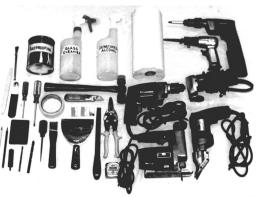
**TOOLS**: marking pencil, tape measure, razor knife, scratch awl, file, fiber stick or plastic squeegee, hand held metal snips, pop-rivet tool, scissors, powered sheet metal shear or other suitable metal cutter, electric drill and bits, cordless screw gun with #2 phillips screwdriver bit
