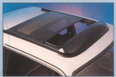
An aerodynamically designed wind deflector improves airflow and reduces wind noise.
