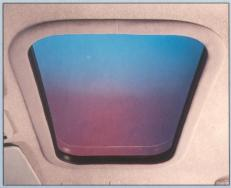
The tempered glass panel slides fully open to provide a clear, unobstructed opening, with no loss of headroom.
