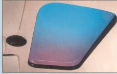
SKYROOF III neatly trims any headliner, hard or soft. Above is a fully trimmed manual model with recessed crank handle. Below, an electric model with optional hard headliner trim.
