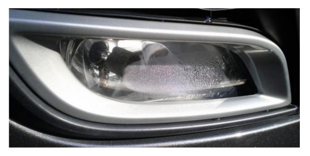
The quick answer to this questions is no. Condensation buildup inside a fog light assembly is normal, and it occurs for a number of reasons. First, vents along the top and bottom of the fog lights housing are necessary to equalize pressure differences that would otherwise cause the entire assembly to crack and fail. Hot fog light bulbs create high pressures inside the fog lights assembly, and temperature differences only increase as lens cover surfaces cool from direct airflow contact at speed.
