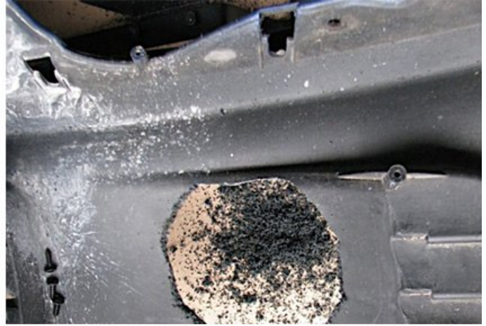
This picture shows the inside of a front bumper that was not originally equipped with fog lights, but has a pre-determined area for mounting them.
