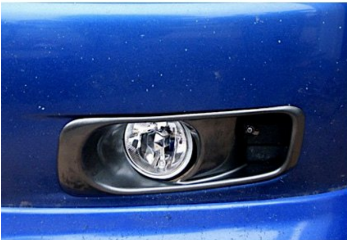
If your vehicle has pre-determined areas for fog lights, surrounding bezel pieces that fit precisely (as seen here) may be available from your vehicle manufacturer or aftermarket suppliers.
