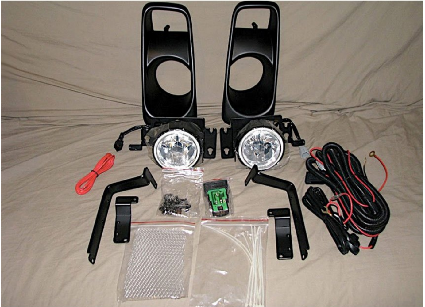
This picture shows the hardware typically included in a universal fog light add-on kit.
